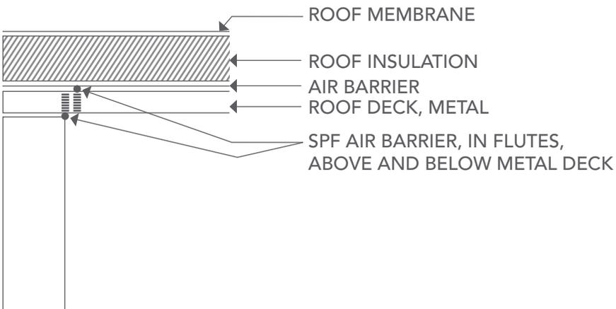
SPF ROOF / WALL INTERSECTION DETAIL: PARAPET WALL
